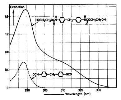
Figure 1. UV spectra of MDI and a urethane from MDI and glycol, both  $6.2 \times 10^{-3}$  eq/liter
