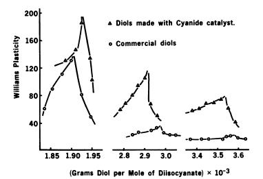
Figure 10. Variation of Williams plasticity of polyurethanes made with diols of various molecular weights; cyanide catalyst used: Zn<sub>5</sub>[Co(CN)<sub>6</sub>]<sub>2</sub> · glyme · ZnCl<sub>2</sub>
