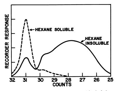
Figure 4. GPC curves of the products separated by the boilinghexane extraction of bisphenol-A oligomer bischloroformates prepared by the aqueous alkaline technique at mole ratio (NaOH: BPA) of 2
