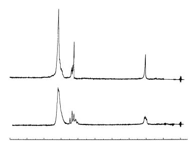
Figure 5. NMR spectra of 1:1 MPP-DPP copolymers; top: blend of homopolymers; bottom: random copolymer from simultaneous oxidation of monomers at 25°C
