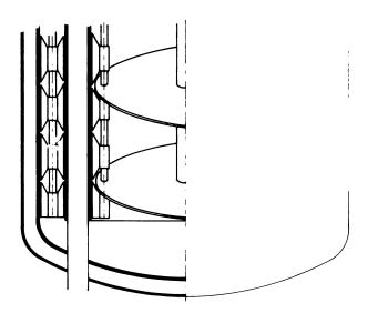
Figure 9. Reactor with cooling cylinder and scraper blades
