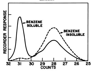
Figure 7. GPC curves for the benzene-soluble and insoluble bisphenol-A oligomer bischloroformates prepared using benzene as cosolvent
