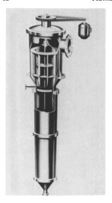
Figure 1. Thin-film evaporator equipped with a fixed blade rotor (Luwa)
