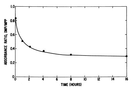
Figure 4. Change in relative intensity of DMP and MPP hydroxyl peaks in infrared spectrum of carbon disulfide solution of homopolymers
