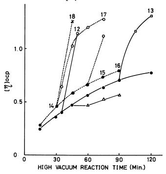
Figure 5. Reaction rates of PET promoted by POC at 275°C and 285°C
