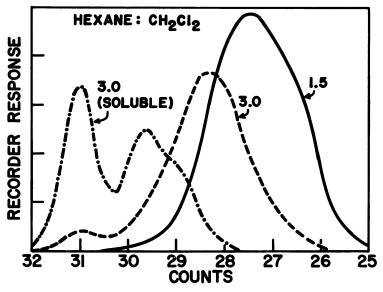
Figure 8. GPC curves of the bisphenol-A oligomer bischloroformates prepared using a 25% excess of phosgene in THF as cosolvent, and fractionated by precipitating from methylene chloride solution by addition of n-hexane. The volume ratios of solvent and nonsolvent are noted
