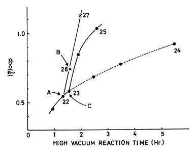
Figure 7. Manufacture of PET by chain extender method on a large scale. Depth of molten polymer: 750 mm. Reaction temperature: 275°-280°C.
