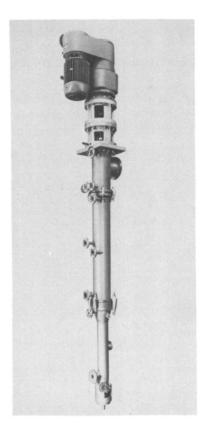
Figure 9. High viscosity machine (Luwa Filmtruder) with rotor drive and discharging device (heating area=0.5 square meter)
