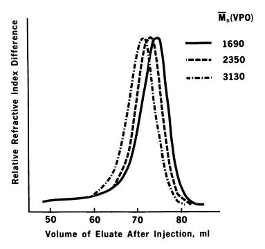
Figure 8. Gel-permeation chromatograms of poly (propylene ether) diols prepared stepwise with  $Zn_s[Co(CN)_6]_2 \cdot glyme \cdot ZnCl_2$
