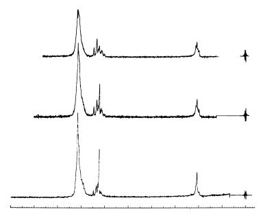
Figure 6. NMR spectra of 1:1 MPP-DPP copolymers; top: random copolymer from oxidation of DPP with MPP homopolymer at 25°C; center: mixed block copolymer from addition of DPP to growing MPP polymer at 60°C; bottom: block copolymer from oxidation of MPP with DPP homopolymer at 25°C
