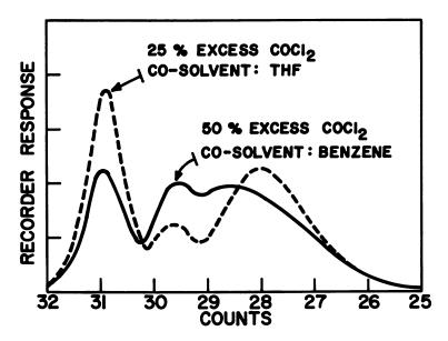
Figure 6. GPC curves of bisphenol-A oligomer bischloroformates prepared in benzene and THF. When the phosgene excess is increased from 11 to 50% with benzene as cosolvent, the molecular-weight distribution is relatively unchanged, compared with Figure 5. However, with THF as cosolvent, a change in phosgene excess from 12.5 to 25% causes a marked change in molecular-weight distribution
