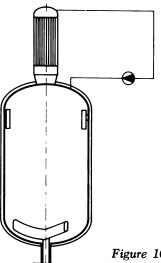
Figure 10. Reactor with reflux cooling and vapor circulation
