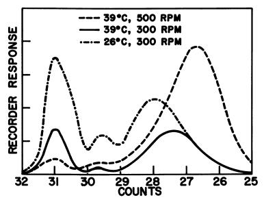
Figure 2. GPC curves for bisphenol-A oligomer bischloroformates prepared by the interfacial technique at the reaction temperatures and stirrer speeds shown
