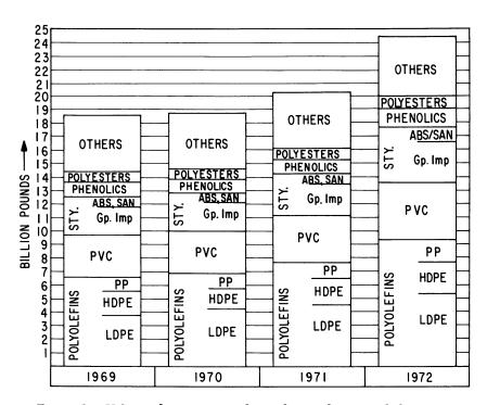
Figure 1. U.S. production of synthetic thermoplastics and thermosets
