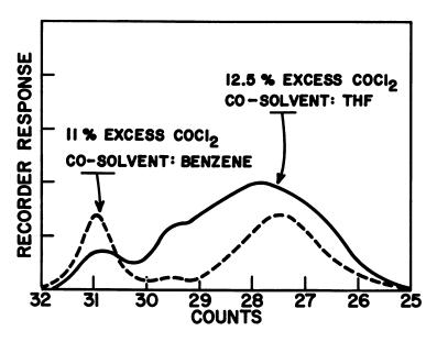
Figure 5. GPC curves of bisphenol-A oligomer bischloroformates prepared in benzene and THF using the same phosgene excess
