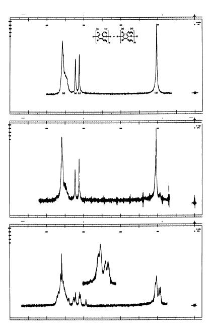
Figure 2. NMR spectra of 1:1 DMP-DPP copolymers; top: homopolymer blend; bottom: random copolymer
