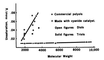
Figure 9. Unsaturation vs. molecular weight for poly(propylene ether) polyols made with Zn<sub>3</sub>[Co(CN)<sub>6</sub>]<sub>2</sub> · glyme · ZnCl<sub>2</sub> and made commercially
