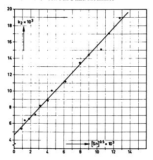
Figure 3. Rate of urethane formation vs. [Sn<sub>o</sub>]<sup>0.5</sup>
