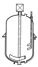
Figure 2. Conventional polymerization reactor with top-driven agitator, baffle, and wall-cooling (volumes up to 40 m³)
