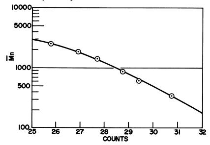
Figure 1. Plot of GPC calibration data showing the relationship of the number-average molecular weight vs. the elution volume (counts) of the particular oligomer
