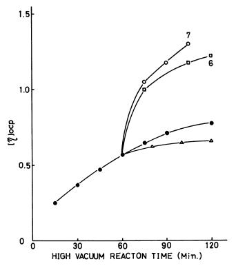
Figure 2. Reaction rates of PET promoted by DPT at  $275^{\circ}C$
