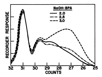
Figure 3. GPC curves for the bisphenol-A oligomer bischloroformates prepared by the aqueous alkaline technique at the mole ratios indicated
