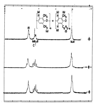
Figure 3. NMR spectra of 1:1 DMP-MPP copolymers; top: homopolymer blend; center: copolymer from oxidation of mixture of monomers at 25°; bottom: copolymer obtained by oxidizing mixture of homopolymers at -25°C
