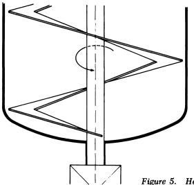
Figure 5. Helical ribbon agitator
