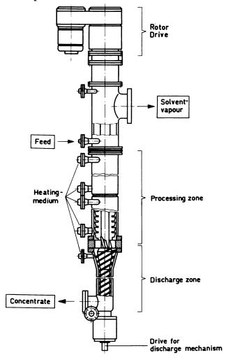
Figure 7. Schematic layout of high viscosity machine (Luwa Filmtruder) with discharge mechanism
